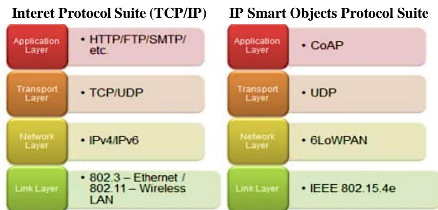
**Figure 2.** TCP/IP Stack and IP Smart Object Protocol Stack (Sutaria & Govindachari, 2013)
