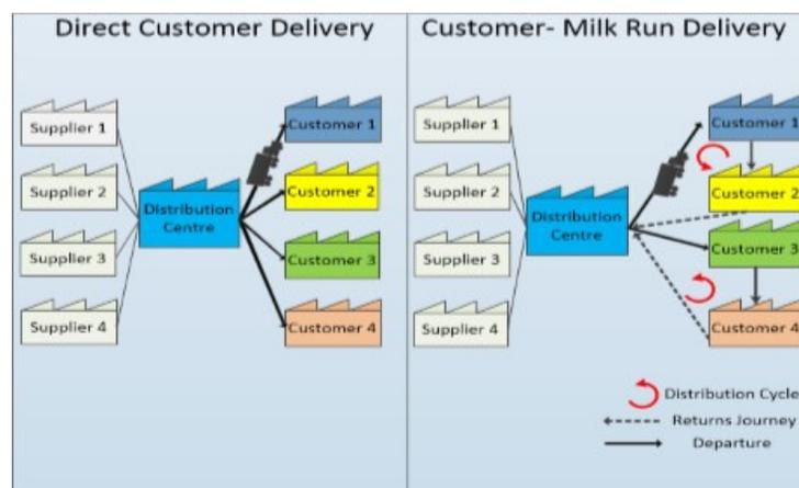
Figure 1. Customer milk run transportation network
